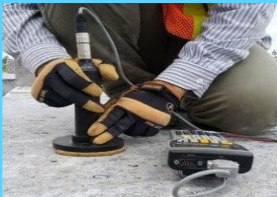
Corrosion Rate Measurement
